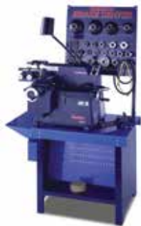
Combination brake lathes for rotors, drums and flywheels
